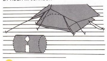
This little radiant heat stove will keep your tent warm, or your duck blind from turning into an icebox. You need a #10 can with both ends cut out and a thick candle about 3" long. Tear all the paper from the can, flatten one side so it won't roll around. Let a few drops of wax melt from the candle onto the inside of the can at the center to form a puddle to set the candle in. The wax will cool and hold the candle firmly.
